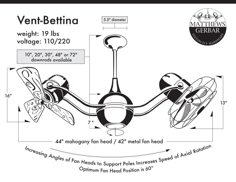
CFM: 4240 (Wood Fan Head) Blade Pitch 19° CFM: 3201 (Metal Fan Head) Blade Pitch 31°
