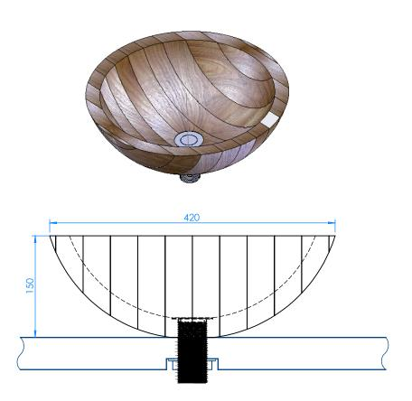
NOTE: IF THE COUNTER TOP IS MORE THAN 35mm (1 1/4") THICK, IT SHOULD BE COUNTERBORED TO RECEIVE THE BRASS LOCK NUT AND LEAVE SUFFICIENT THREAD FOR THE WASTE FITTING
